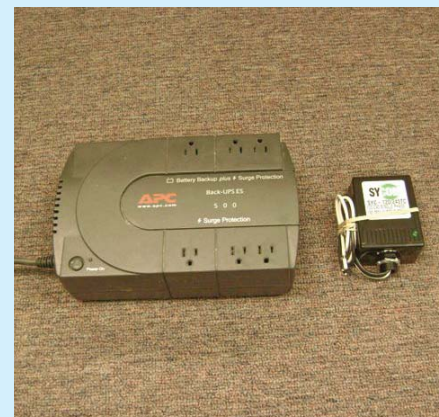
Examples of surge protectors are (L) Surge protector with battery backup and (R) Whole house surge protector.
