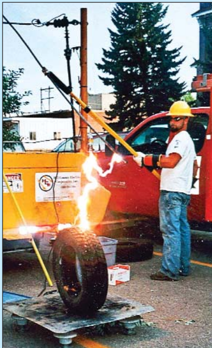
At an HRDC Kids Fair, lineman Curt Olson demonstrates how an automobile tire conducts electricity.
