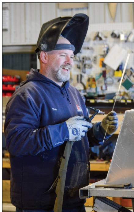
From left: Brett Nienhuis welds aluminum. All “Big Fish” drift boats are 100-percent welded; Nienhuis demonstrates his handicap-accessible boat; “The Patriot” is his favorite custom drift boat. Boat photos courtesy of Brett Nienhuis.
